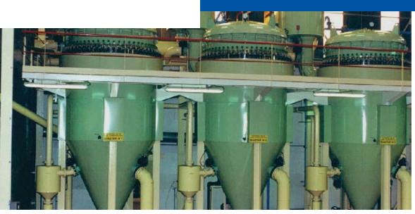
SOLAFT<sup>®</sup> Back Flush Filters for Diastar<sup>™</sup> Vertical Pressure Leaf Filters are a leading high-quality product in the Micronics Engineered Filtration Group's Liquid Filtration product range. They are ideally suited to the demands' of today's alumina industry from Brazil to Australia, where our team has extensive, long-standing technical expertise and application knowledge.
