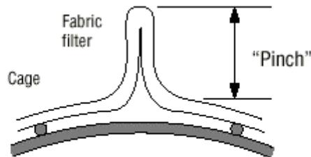
Figure 2. "Pinch" is calculated by subtracting the actual cage circumference from the bag circumference; then dividing the result by 2.
