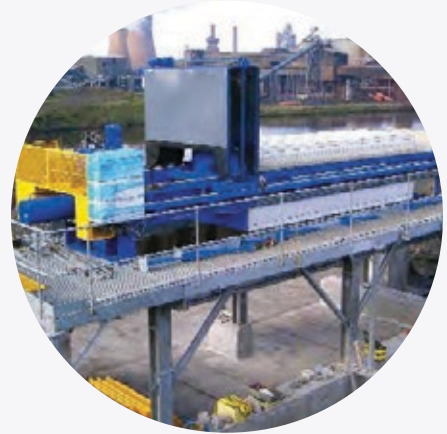
Complete refurbished filter. Addition of booth washer and support structure.
