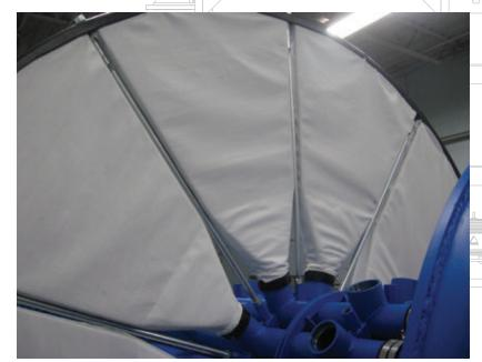
Efficient disc sector and center barrel design to maximize the hydraulic throughput & achieve low cake moisture
