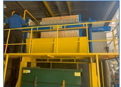
Footprint was an issue in the facility so we carefully examined the tradeoffs of different size/capacity presses, e.g. a 1000mm, 25 ft<sup>3</sup> press vs a smaller capacity press with a larger stack of filter plates. We determined that a 1000mm, 25 ft<sup>3</sup> filter press would best address their space issues and allow them multiple operating advantages.
