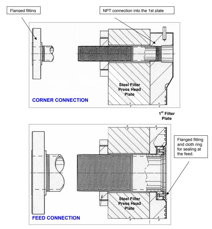
The drawings show common methods for feed plate connections. In some cases NPT threads are used to connect the Head (1<sup>st</sup>) plate. Another method uses a 1" connector plate, either flanged fittings into counter bored holes or NPT threads create the seal. Contact Micronics if you need additional help with your filter press or plate set up.
