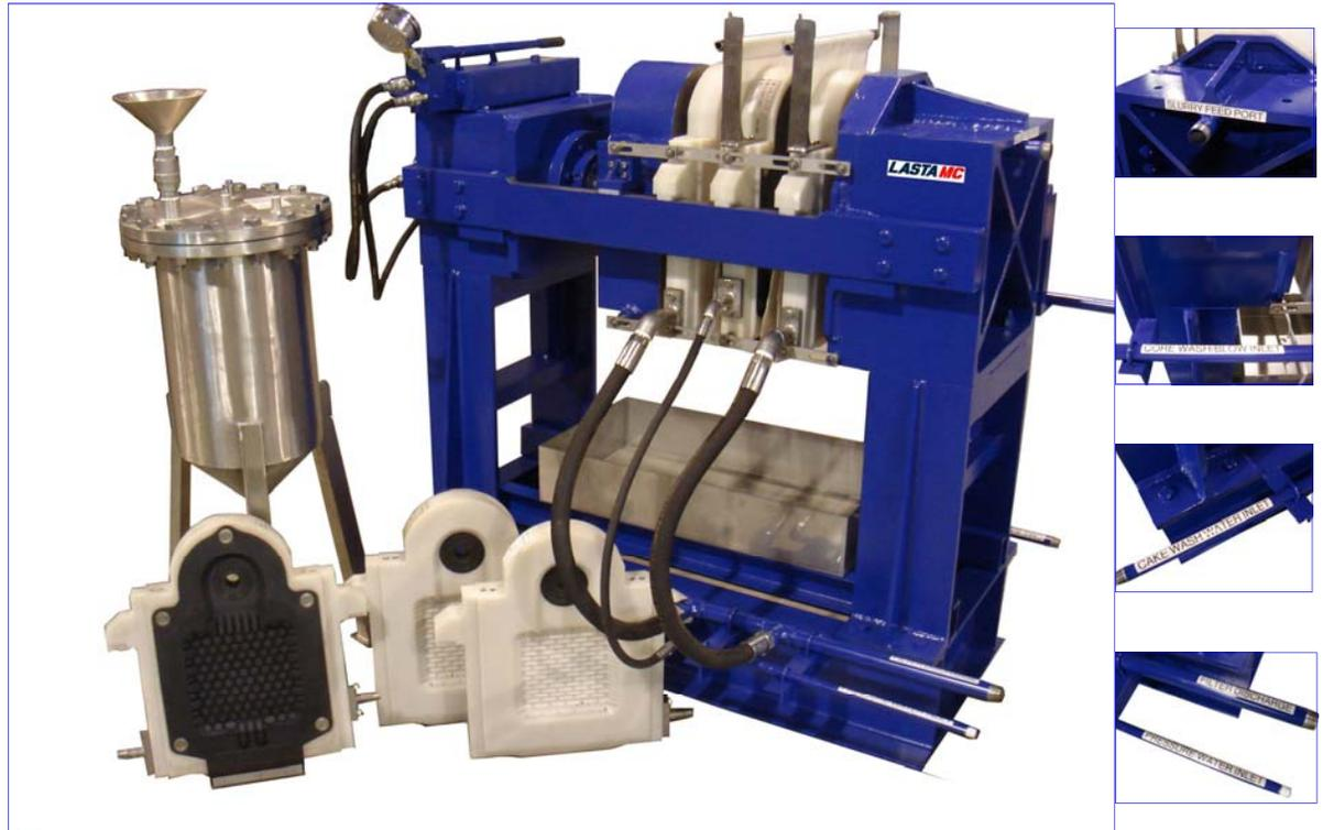
**A SELF CONTAINED TEST UNIT:** FILTRATION FEED PRESSURE TO 7 BAR (100PSI), SQUEEZE PRESSURE TO 20 BAR (295PSI), CAKE WASHING, CORE WASH/BLOW, CAKE AIR DRYING, CAKE MOISTURE ANALYSIS, CAKE THICKNESS CAPABILITY OF 30, 40 AND 50MM USING EITHER A RECESSED PLATE OR MIXED PACK MEMBRANE CONFIGURATION.
