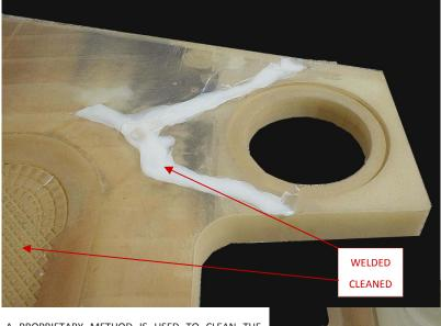
AGGRESSIVE MINE TAILINGS AND CONCENTRATE APPLICATIONS FREQUENTLY RESULT IN DAMAGED PLATES CAUSED BY EXCESSIVE AIR BLOW DOWN AND/OR FAILED FILTER CLOTHS, WHICH ALLOW THE FEED SLURRY TO SCOUR THE PLATES. DIFFERENTIAL FEED PRESSURE CAN ALSO CAUSE WARPING AND CRACKING OF THE FILTER PLATES.
