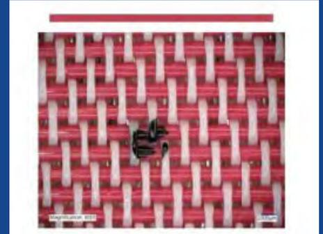
NFM® Blue-Flexx™ design provides increased belt structural integrity due to the fabric's interlocking weft yarn strands
